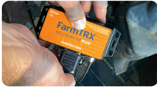
Yield Monitor ECU connection via 15 Pin connector
