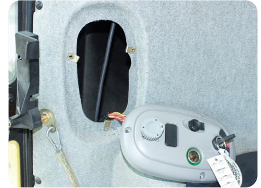
Routing of Primary Wiring Harness along inside of door post with ignition switch assembly removed for access
