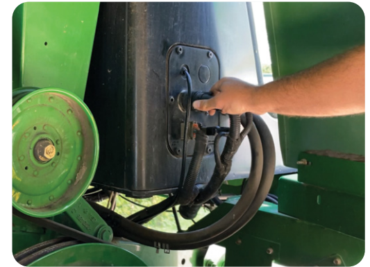
Routing of Primary Wiring Harness along inside of door post with ignition switch assembly removed for access
