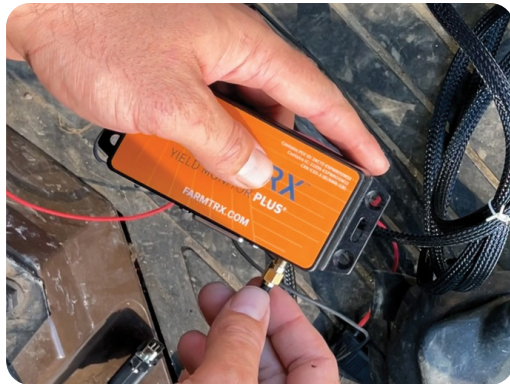
Yield Monitor ECU connection via 15 Pin connector
