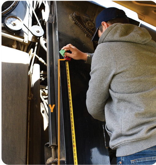
Height (Y) from the center of the bearing to the center of the drill hole
