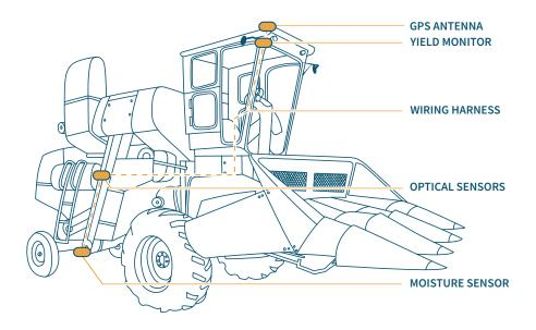
GPS Antenna—The external multi-constellation antenna is connected to the Yield Monitor via an SMA connector and mounts on the roof of the cab on the centerline of the combine.
